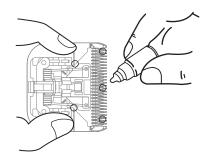
${f S}$  Do not detach the blade spring while maintaining to avoid malfunction.
